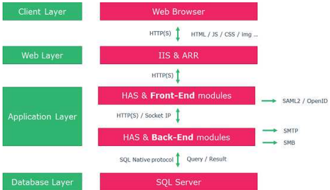
Figure 4 HAS Communication Stack
